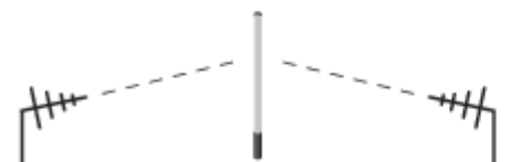
Antennas not on the same level plane
