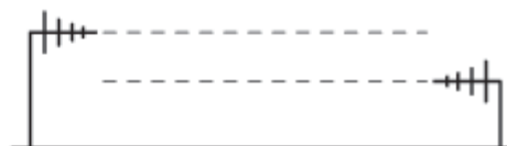
Antennas not aligned
