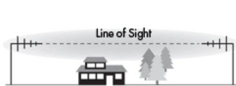
Obstructions in the lobe of the radio signal
